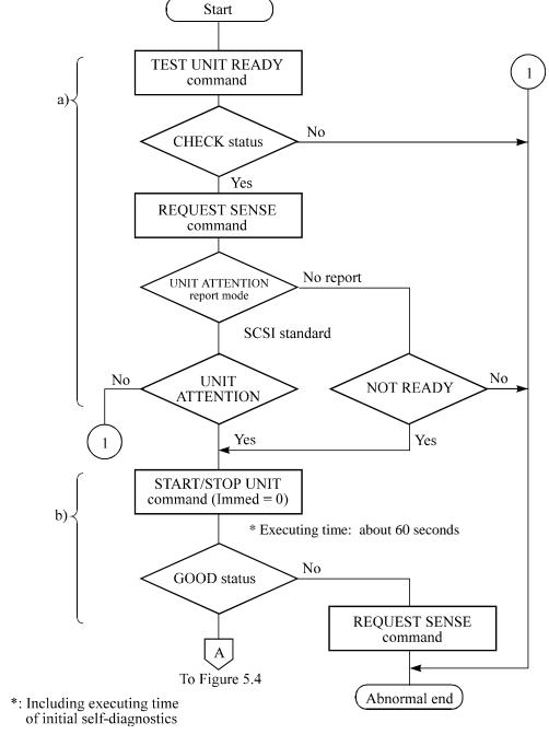
Figure 5.5 Checking the SCSI connection (B)
